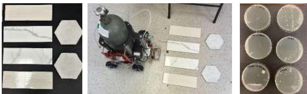
Fig1. Floor tiles, Plasma Hoover, and Bacteria colonies with and without Plasma Exposure
