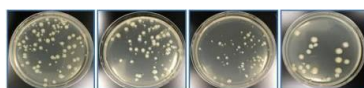
Fig 2. Raw data from a stage four serial dilution, from L to R: Control, argon plasma with nitrogen, and argon plasma
